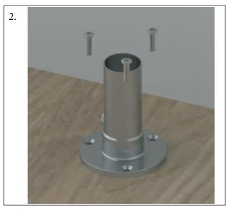
Attach false leg to the floor, ensure the false leg is in the correct location. For dual fuel models esure that the incoming water feeds are located correctly.
