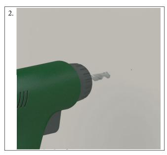
Ensure that there are no wires or pipes behind the marked locations for the fixings. Drill holes for fixings.
