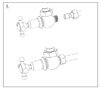
Attach the feed pipes to the radiator valves using the compression olives and nuts.
