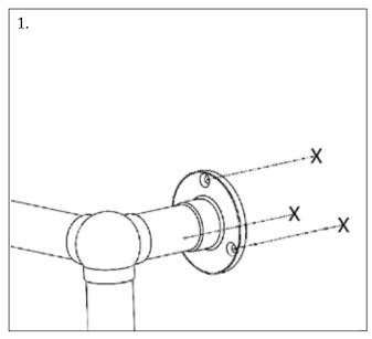
After the towel rail has been thoroughly inspected and carefully unpackaged measure the fixing points on the wall and floor, ensuring that the rail is level and aligned with the incoming feeds or electric supply where applicable. Whilst every effort is made to maintain the orientation of each foot, we cannot guarantee this, therefore it is imperative that each screw position is marked out before assembly.
