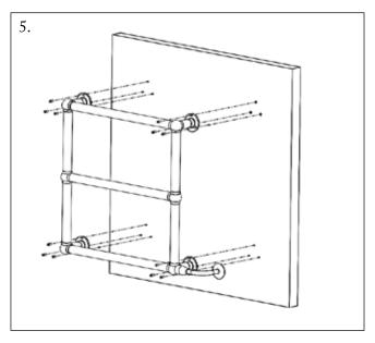
\*Applicable to electric model. Attach the rail to the wall using the wall plugs installed in section 1.
