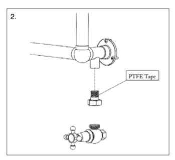
Fit the radiator valve tail thread using an appropriate allen key, use an appropriate PTFE tape on the thread. DO NOT OVER TIGHTEN. Then loosely attach the radiator valve.
