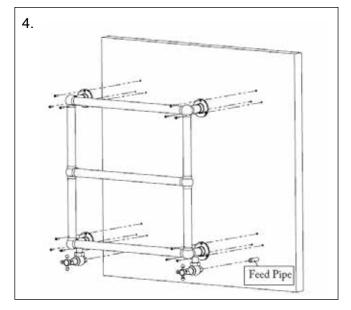
Attach the rail to the wall using the wall plugs installed in section 1.
