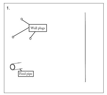
Ensure that the 15mm feed pipes are aligned correctly for fitting to the radiator valves. For the best fitting we recommended that approximately 16mm of pipe is proud of the wall and each pipe is located approximately 85mm directly below the center point of the lower foot.
