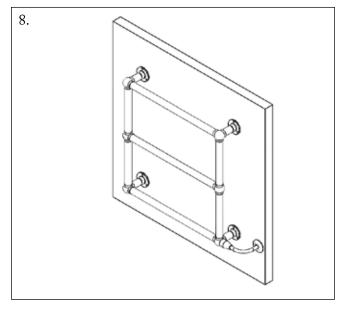
For electric models, test the rail. IMPORTANT: Electric elements should be fitted only by a suitably qualified electrician and must be earthed and connected to a cable outlet in the bathroom in accordance with I.E.E wiring regulations. The electrical connection should be made to a 5-amp fused fixed spur located outside the bathroom.
