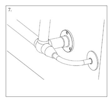
Connect the cable to the element in the towel rail then fit the shroud to the towel radiator.
